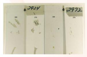
After being recoated with urethanes, these panels were exposed to 100% humidity for one week. Adhesion was evaluated with a knife.
