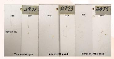
Panels of Devran® 223 were aged for the above stated time periods and were recoated with aliphatic urethane enamels. The recoated panels were then exposed outside for one year. Adhesion was evaluated with a knife.
