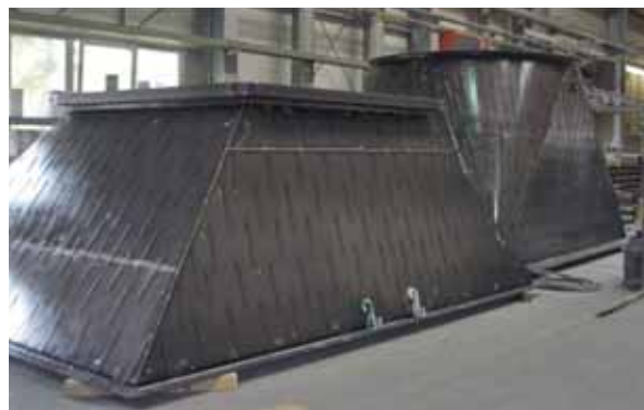
Flue gas ducts and hoods
