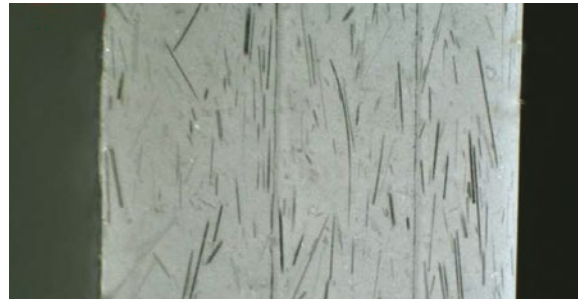
Coating cross-section showing flake orientation
