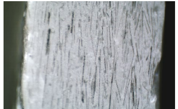
Coating cross-section showing flake orientation
