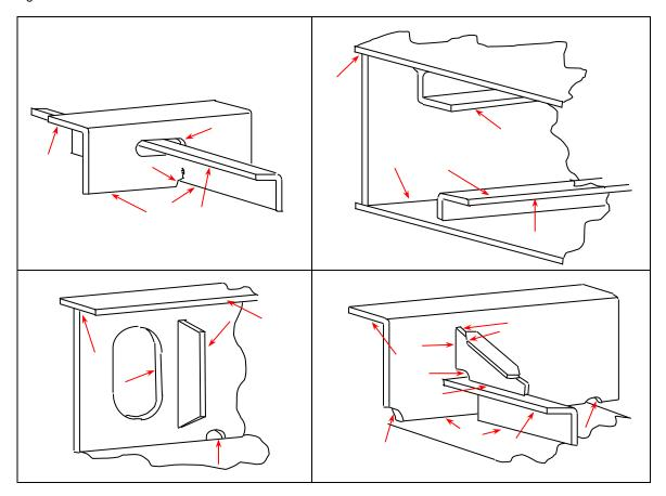
In general, stripe coats should be applied by brush. Application by roller should be limited to the inside of scallops. In exceptional circumstances, it may be acceptable to apply a stripe coat to the backs of angle bars by narrow-angle spray.
