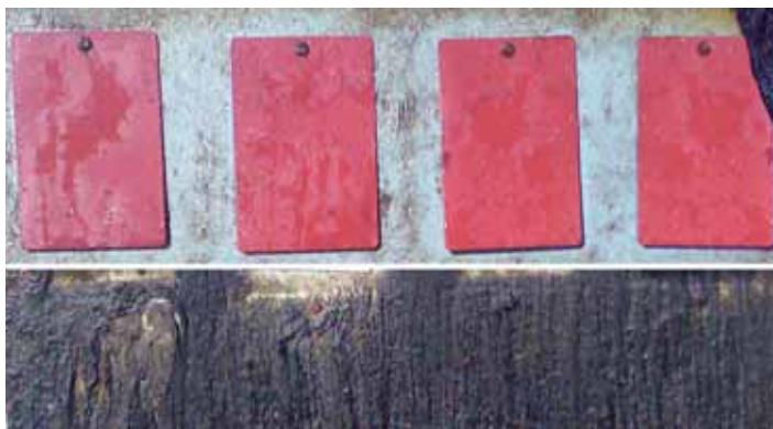
Intersleek® 970 panels (top); Anti-corrosive panels (bottom) after immersion in sea water for six months
