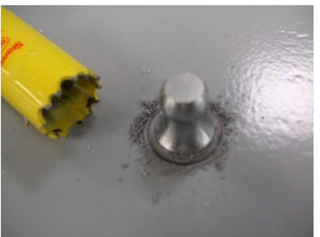
Attach the tensile tester, taking care that it is perpendicular to the substrate, i.e. that no bending force will be introduced. Apply tensile stress, uniformly increasing at a rate not greater than 1 MPa/s. Record the tensile stress to failure and examine the fracture surfaces. If failure is mainly associated with the adhesive, repeat the test using a more suitable adhesive.
