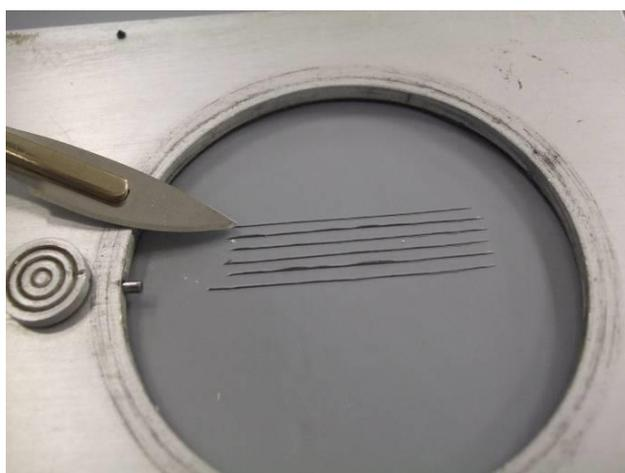
Rotate the panel and make a further six cuts, crossing the original cuts at 90° to form a square lattice pattern.
