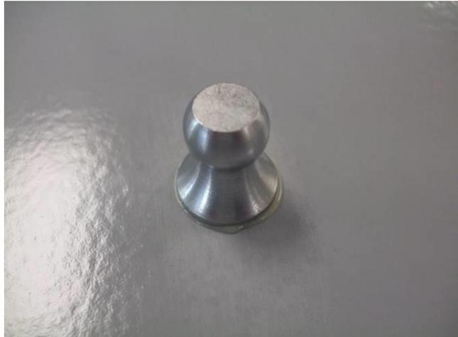
Allow the adhesive sufficient time to cure, minimum 24 hours. Carefully cut through the coating, to the substrate, around the circumference of the test cylinder. If results are required without cutting through the coating, this must be reported.
