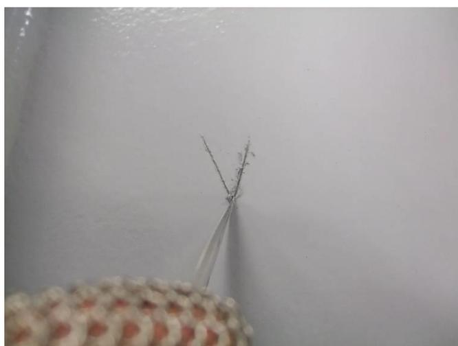
Inspect the V cut to confirm that it has penetrated through the paint films to the substrate: if not, carefully repeat the cutting action where penetration is insufficient, keeping in mind that this may affect the adhesion along that incision and result in a lower assessment.
