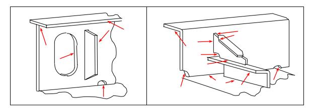
In general, stripe coats should be applied by brush. Application by roller should be limited to the inside of scallops.
