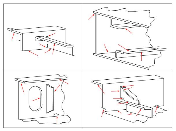
In general, stripe coats should be applied by brush. Application by roller should be limited to the inside of scallops.
